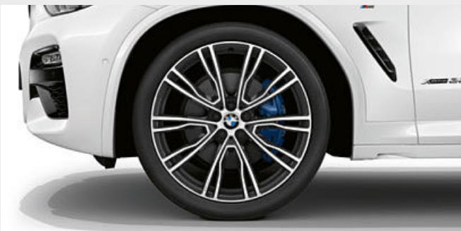
□ 21" BMW Individual light alloy wheels V-spoke style 726 I in Bicolour Orbit Grey, gloss-lathed, with mixed tyres and run-flat properties, front 8.5J x 21 with 245/40 R21 tyres, rear 9.5J x 21 with 275/35 R21 tyres.
