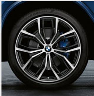
○ 21" BMW M light alloy wheels Y-spoke style 701 M Bicolour Black matt, gloss-lathed on the visible side. Complete summer wheel set with mixed, run-flat tyres. Front tyres: 245/40 R21. Rear: 275/35 R21.
