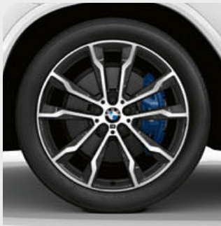
□ 20" M light alloy wheels Double-spoke style 699 M in Bicolour Orbit Grey, gloss-lathed 1,2,* , with mixed tyres and run-flat properties, front 8J x 20 with 245/45 R20 tyres, rear 9.5J x 20 with 275/40 R20 tyres.
