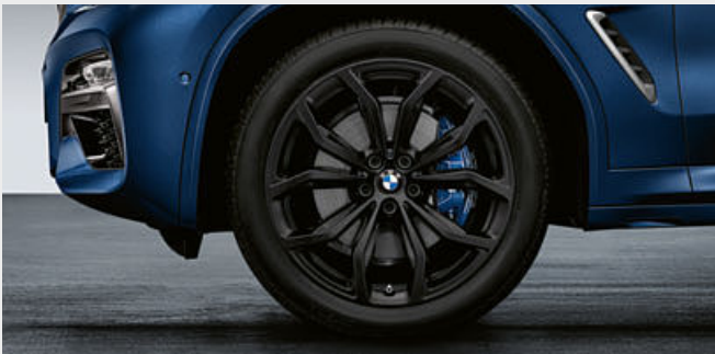
○ The high-quality 20" light alloy wheels Y-spoke style 695 are in matt Black and feature spokes arranged on two levels. Complete summer wheel set with mixed, run-flat tyres. Front wheels: 8J x 20 with 245/45 R20 103W XL RSC tyres. Rear wheels: 9.5J x 20 with 275/40 R20 106W XL RSC tyres. Also available as a complete winter wheel.
