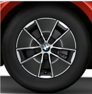
□ 16" light alloy wheels turbine styling 773, Bicolour Orbitgrey, BMW Efficient Dynamics, gloss-lathed, wheel size 6.5J x 16, 205/60 R16 tyres.*
