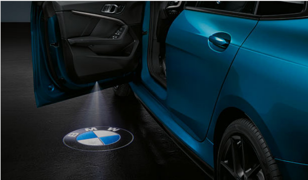
○ The LED door projectors are activated when the doors are opened. They project an image onto the ground next to the car using an interchangeable slide.
