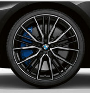
□ 19" M light alloy wheels Double-spoke style 552 M Bicolour Jet Black, gloss-lathed, wheel size 8J x 19 with 235/35 R19 tyres.⁵*
